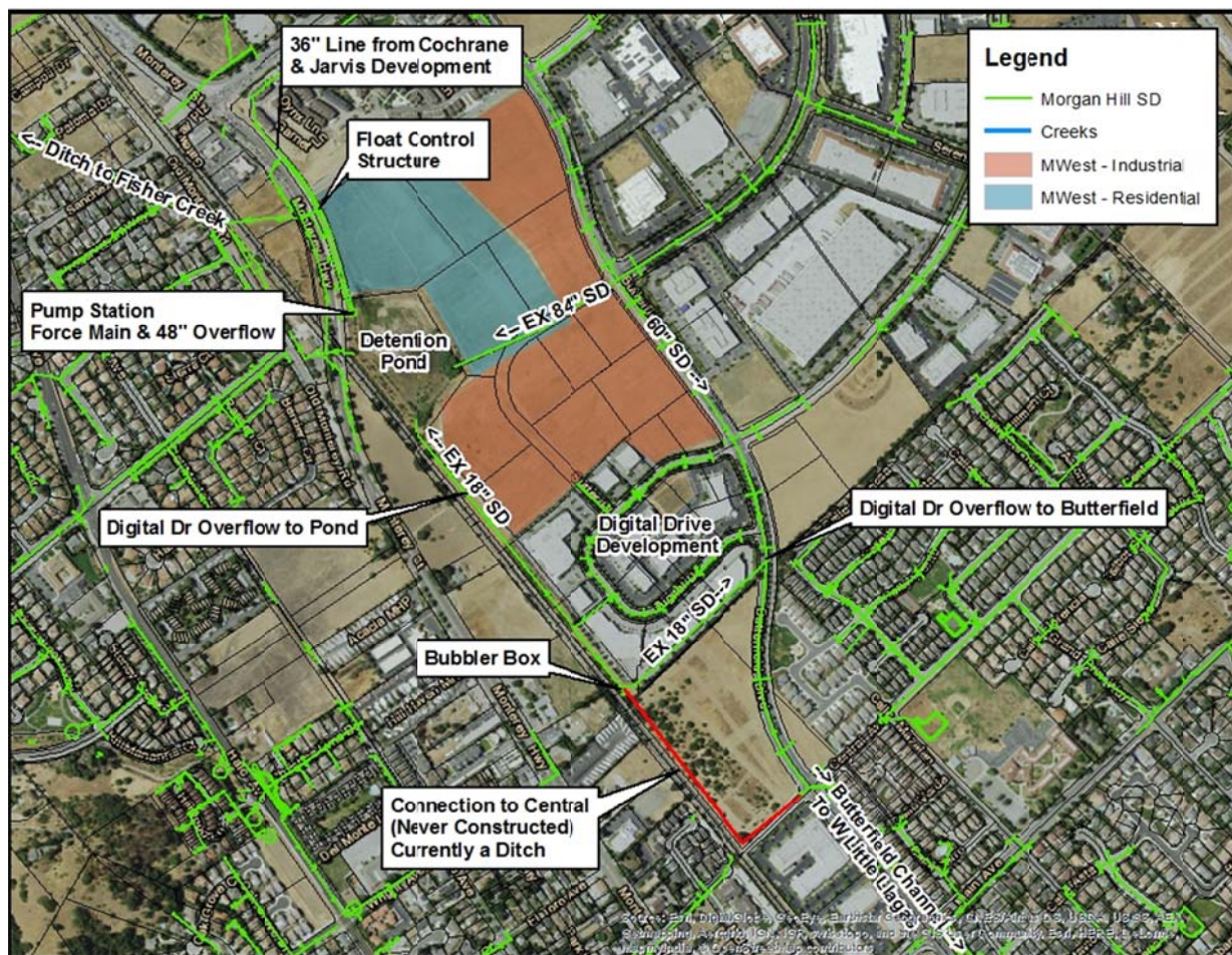
Figure 1: Detention Pond System Layout
