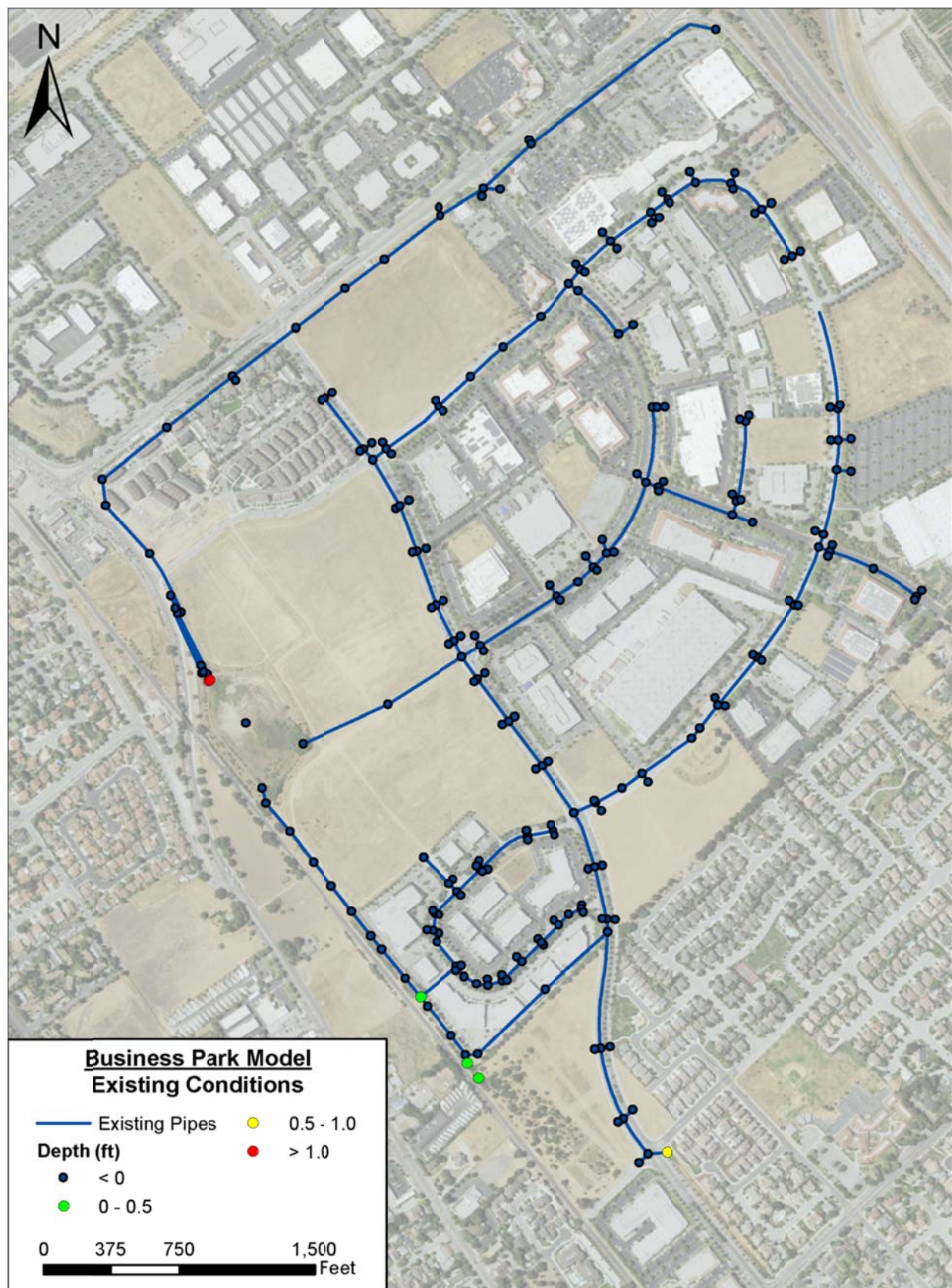
Figure 3: Existing System 10-year Hydraulics with Blockages Removed.
