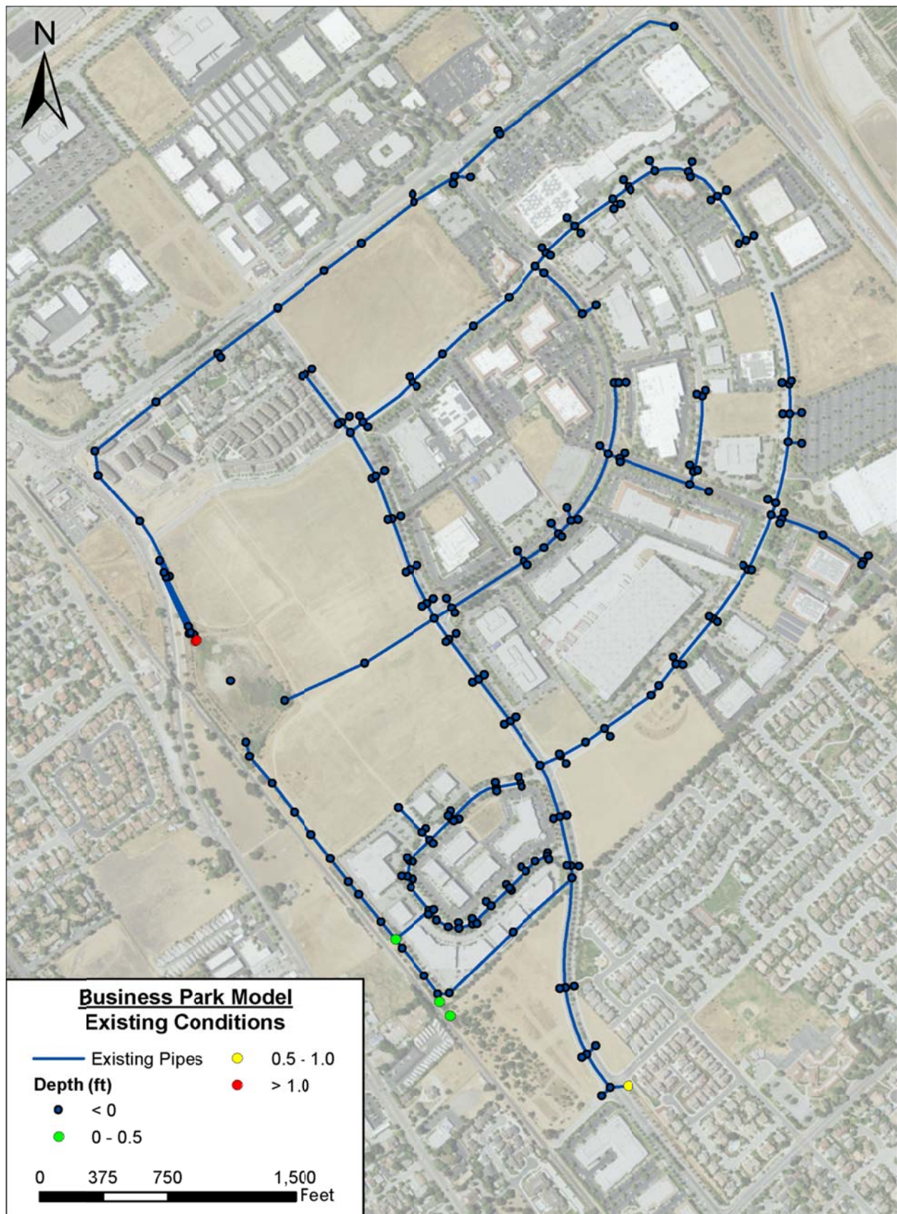
Figure 3: Existing System 10-year Hydraulics with Blockages Removed.
