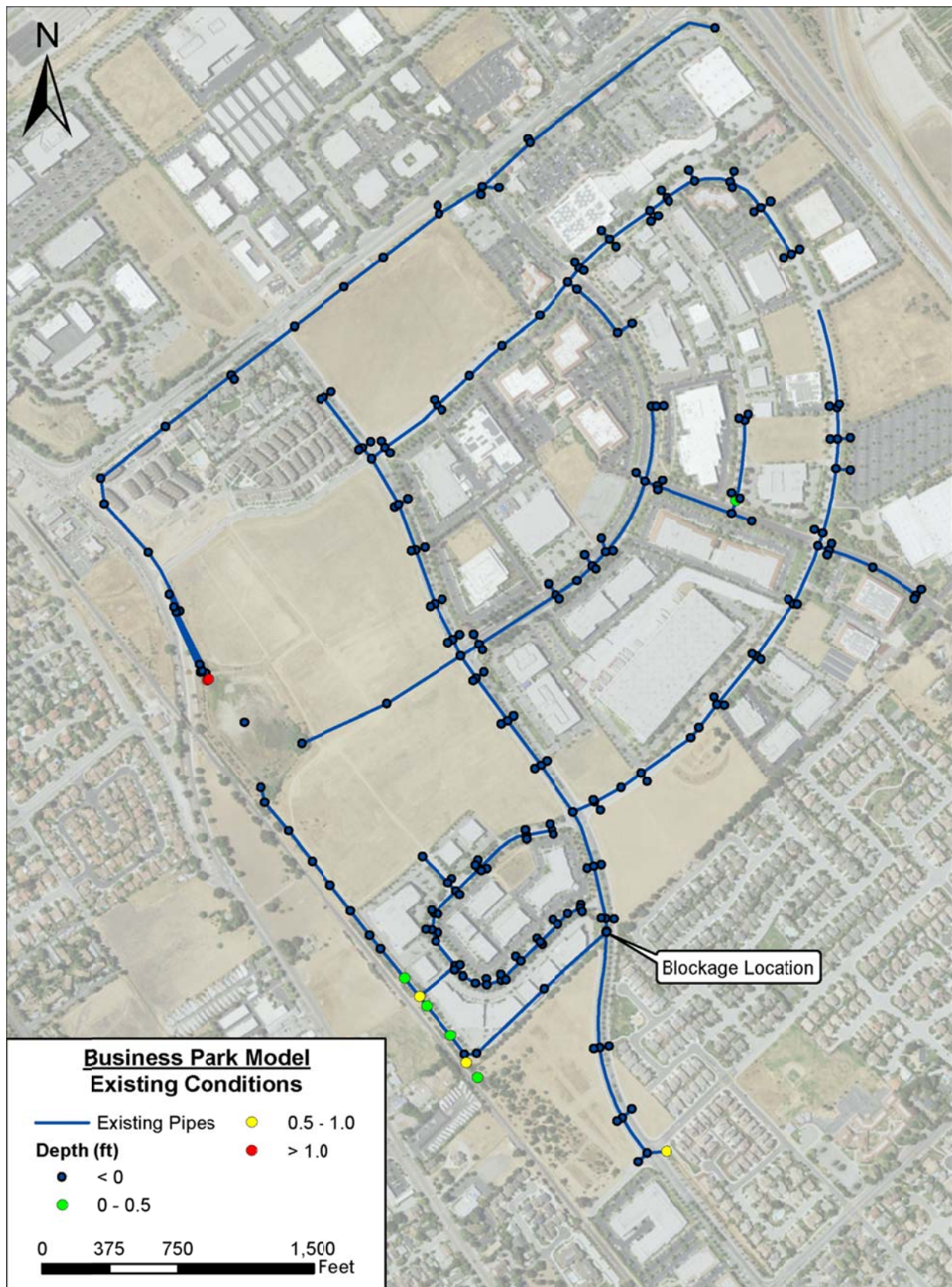
Figure 2: Existing System 10-year Hydraulics
