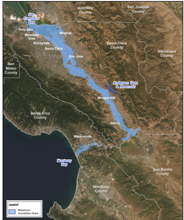
Maximum Flood Area from Anderson Dam Failure
