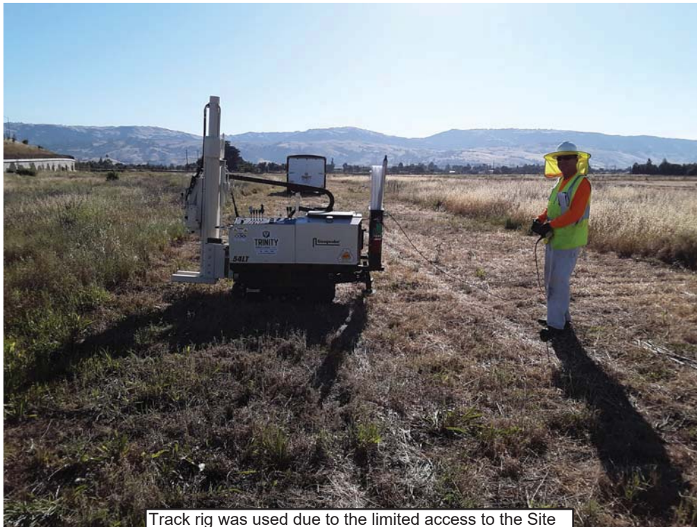
Track rig was used due to the limited access to the Site
