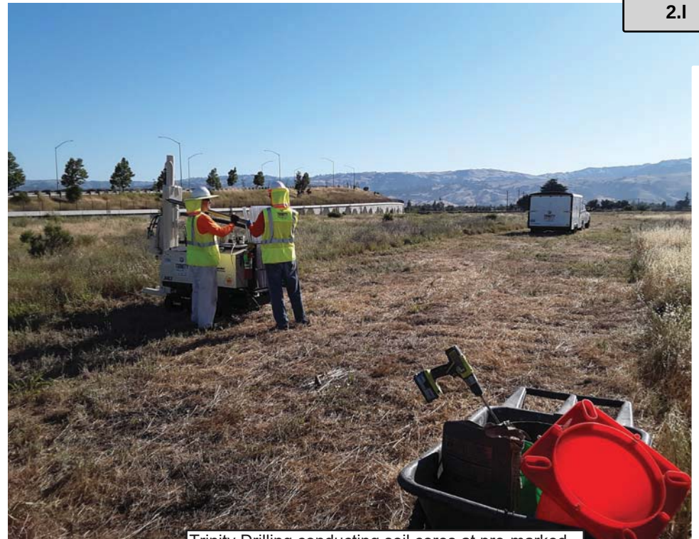
Trinity Drilling conducting soil cores at pre-marked locations with hydraulic driven probe track rig.
