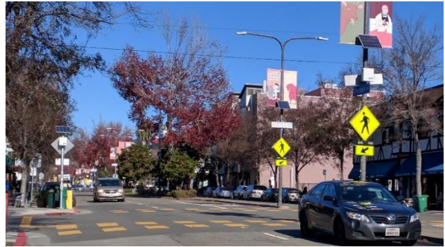
Figure 3-3: Example of rectangular rapid flashing beacons (RRFBs)
