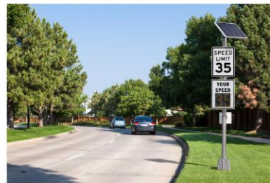
FIGURE 52 Pole-mounted Radar-Speed Sign (Source: Tim Magee)
