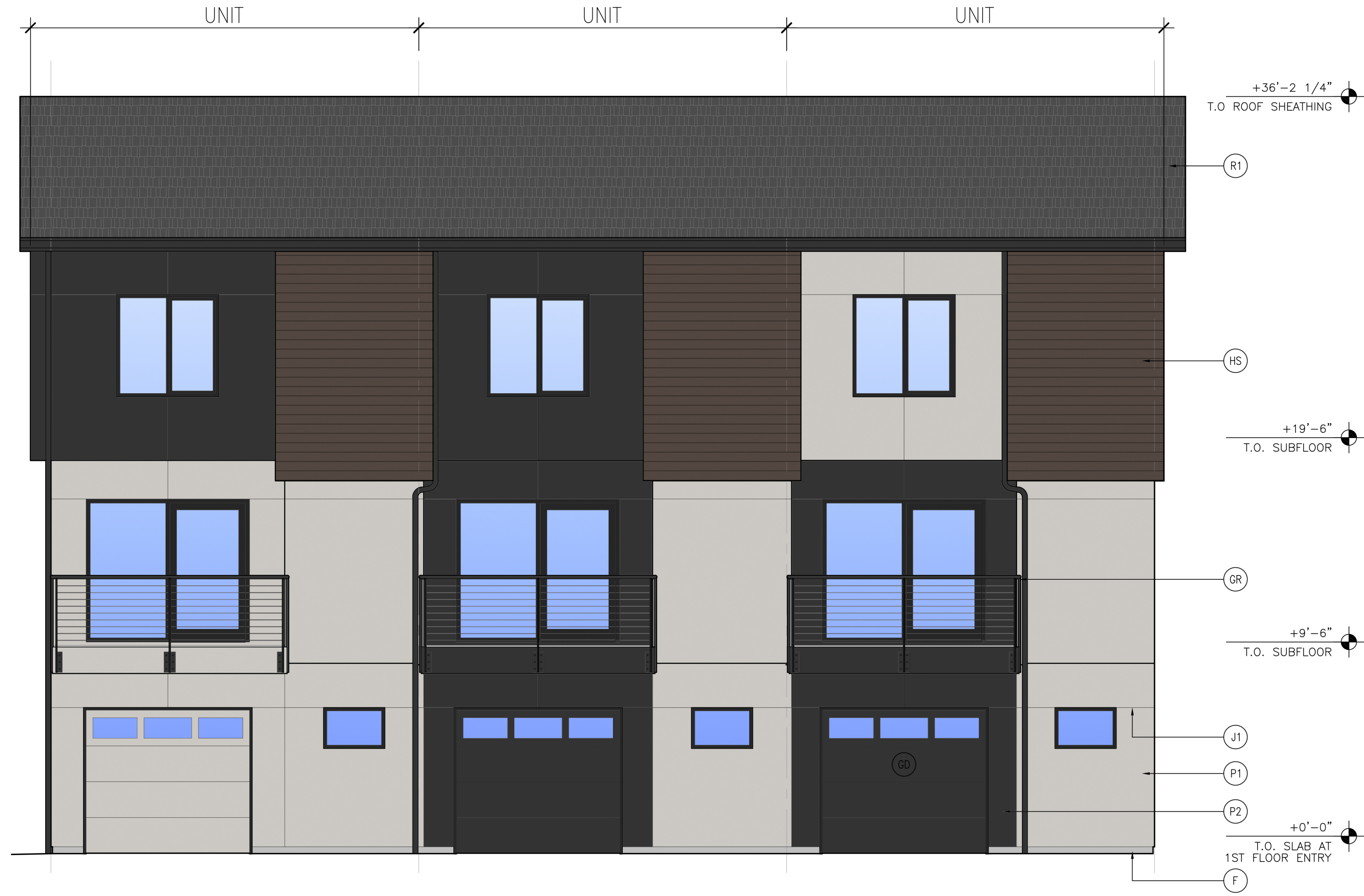
BUILDING 1 - NORTH / STREET ELEVATION SCALE : 1/4" = 1'-0"
