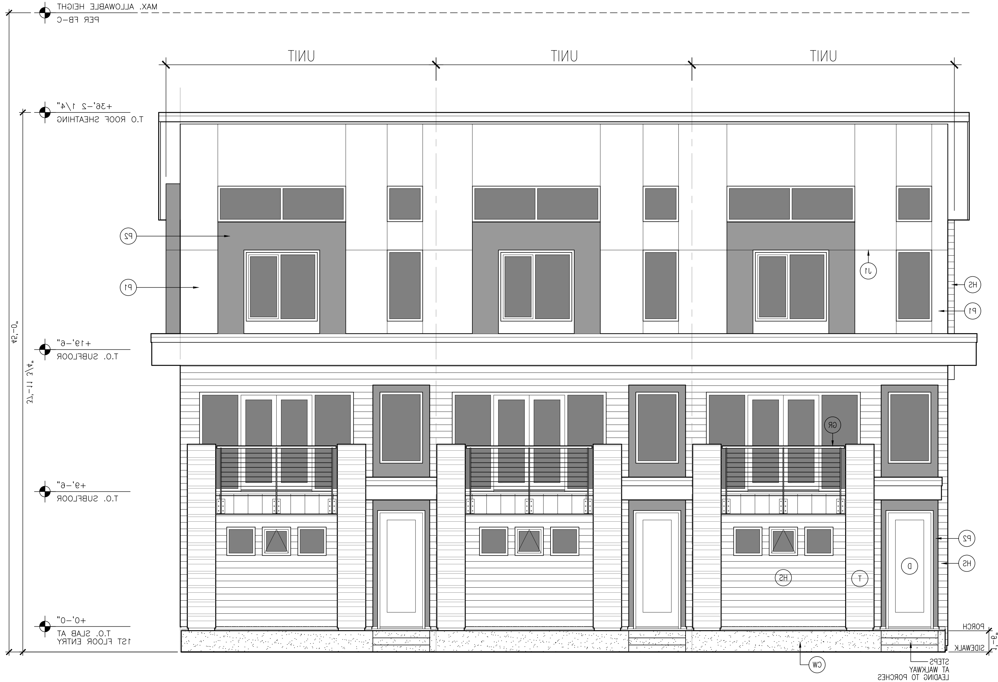
BUILDING 2 - NORTH / STREET ELEVATION
