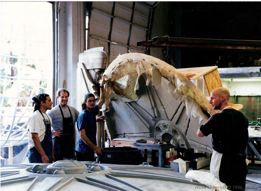
Building and molding the 'Edgar Bug' spaceship for Men In Black 1999 – ILM Modelshop
