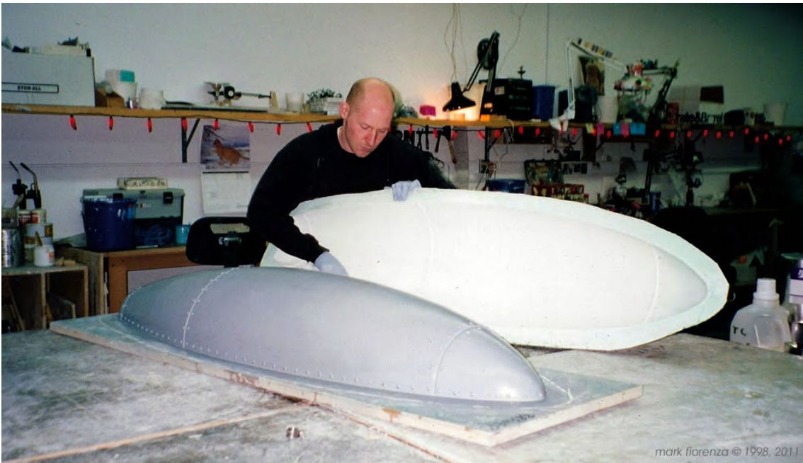
Casting large scale fiberglass rocket for Cool Rockets custom rocket models & props
