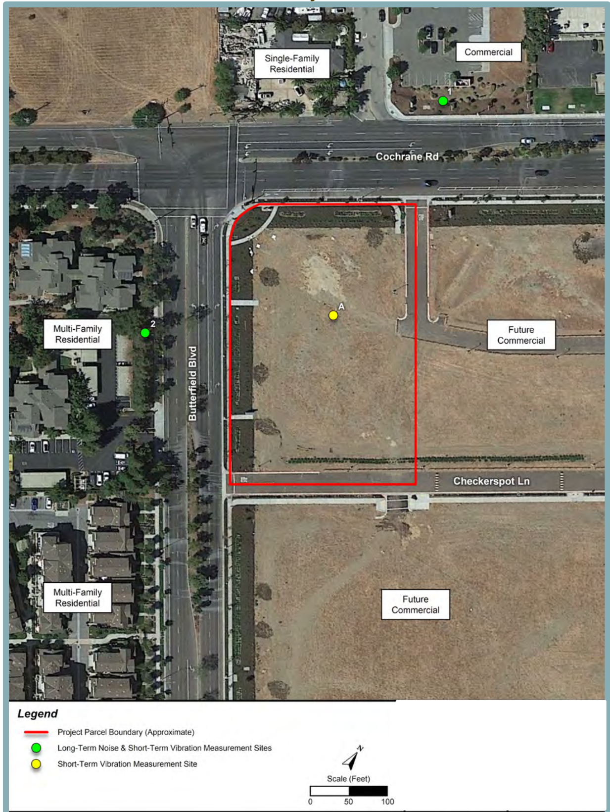
Figure 8 Noise Survey Locations
