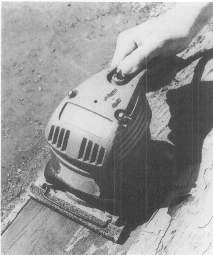
Fig. 11 The orbital sander can be used for limited paint removal, i.e., for smoothing flat surfaces after the majority of deteriorated paint has already been scraped off. Photo: Charles E. Fisher, III.
