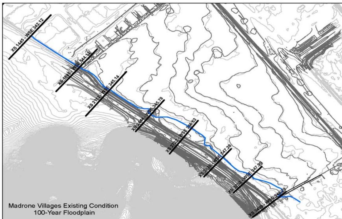
Figure 14. Existing Condition Floodplain on Project Site, 100-Year Storm
