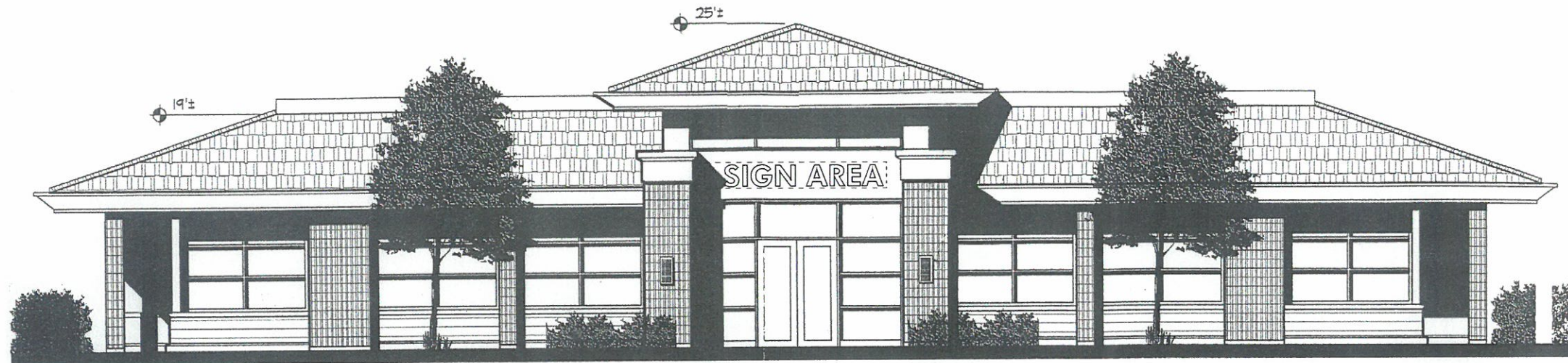
T-D Elevation - 18" internally illuminated pan channel letters mounted on bldg.fascia - Major Pad & Single Occupant Pad Tenants Scale: 3/32" = 1'-0"
